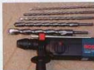
Masonry bits feature a chisel-like tungsten carbide tip and are often used with a pumping action to pull chipped material out of the hole.
