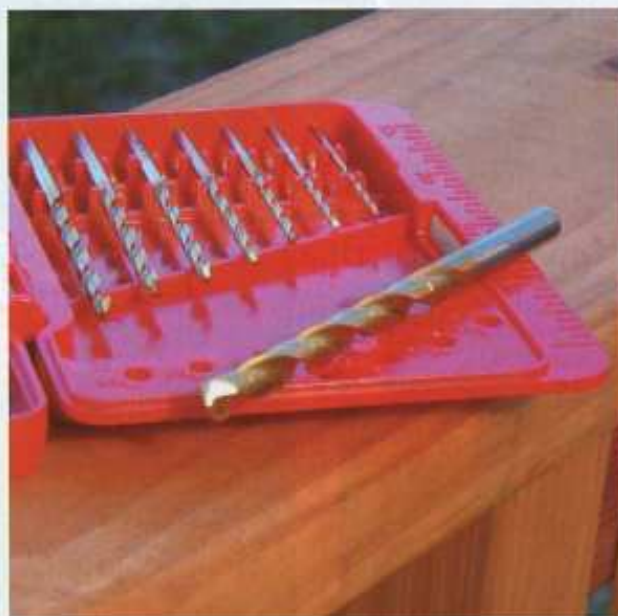
Modern materials and advanced designs make the today's drill bits more efficient than ever. Shown are Vermont American's Titanium-coated twist bits. The titanium coating lasts six times longer than standard high-speed steel bits.
