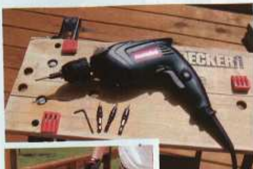
Adjustable pilot bits pre-drill screw holes to prevent splitting wood. They can also countersink screw heads flush with the wood surface.
